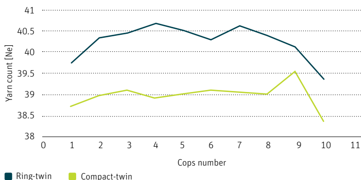
Fig. 21 The loss of good fibres is smaller with the compact twin technology compared with the conventional ring spinning twin technology
