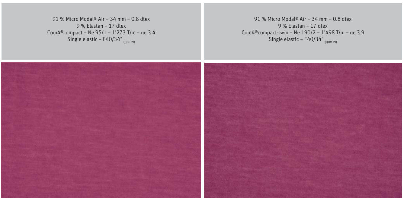
Fig. 45 The knitted fabric made of twin yarn (right) shows a more uniform appearance than of single yarn (left)
