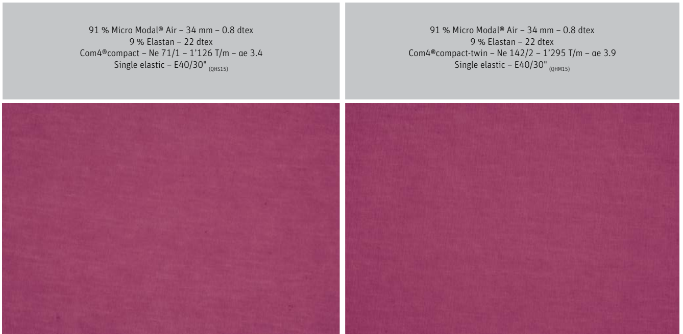
Fig. 44 The knitted fabric made of twin yarn (right) shows a more uniform appearance than of single yarn (left)
