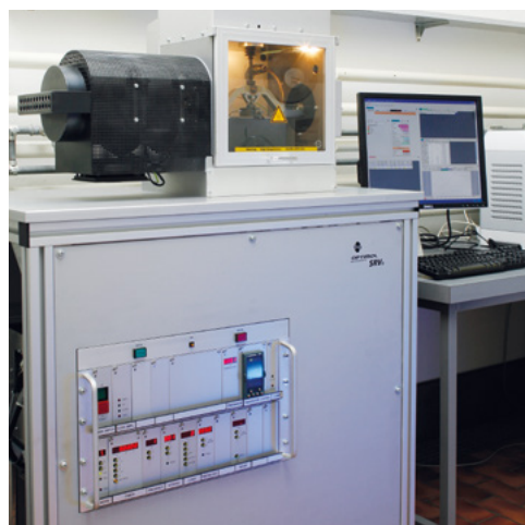
Fig. 3: Tribometer at IMPE in Winterthur
