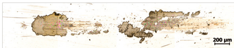
Fig. 5: Contact surface of ring material after tribological testing
