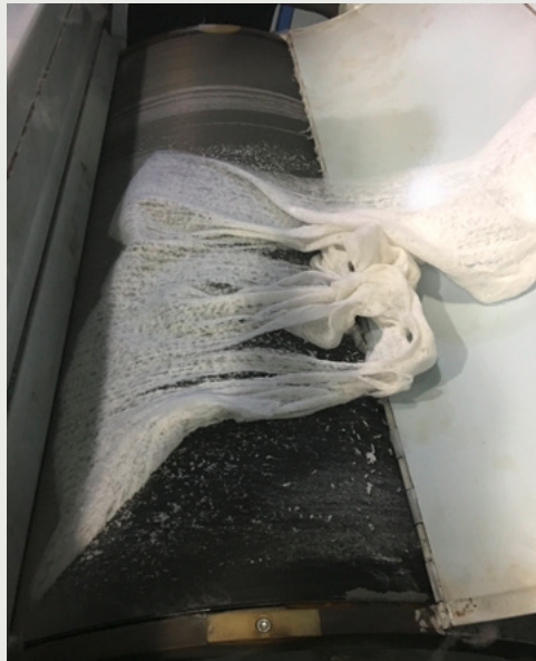
Fig. 6: Choked doffer at customer's site, requiring cleaning every other day
