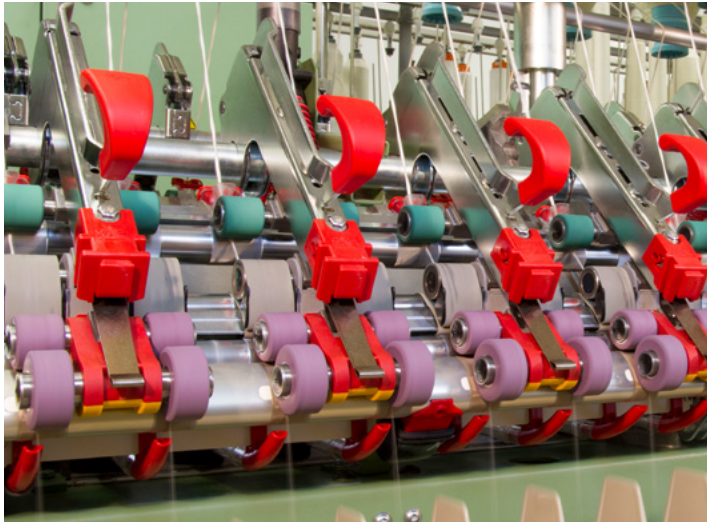
Fig. 1: HP-GX 3010 Top Weighting Arm, here with EliTe ® Advanced Compact Spinning System
