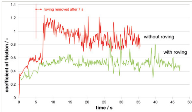
Fig. 4: Coefficient of friction with and without cotton fibres
