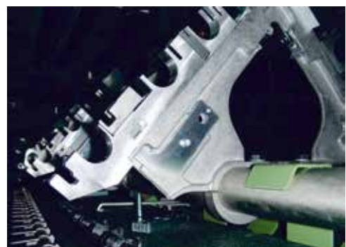
Fig. 9 - Remachining of existing roller stand
