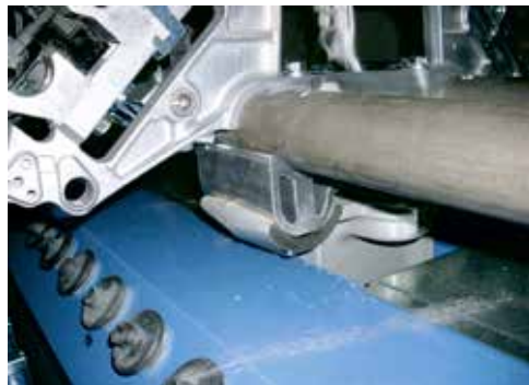
Fig. 5 - Use of spacer rails
