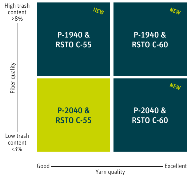
Fig. 2: Application areas for the card clothing sets
