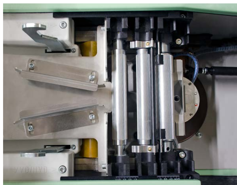
Fig. 4: From a short-fiber content of 27% and above when using virgin cotton, two drafting zones are essential.
