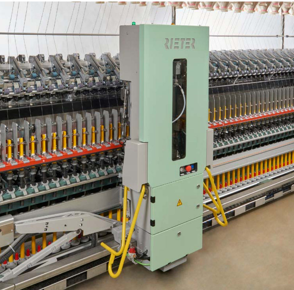
Fig. 1: The piecing robot ROBOspin increases productivity and also reduces personnel costs.
